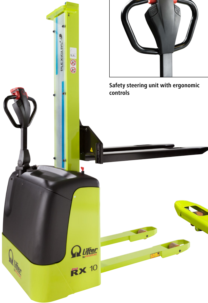
Accessible passageway width: 2210 mm for 800 x 1200 mm pallets, lengthwise entry
