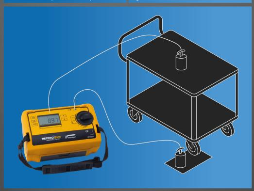
The test is carried out in accordance with IEC 61340-2-3 and meets the requirements of IEC 61340-5-1.
