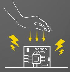
These charges discharge upon contact with the component, and can damage it. Resistance ranges are defined in accordance with IEC 61340:2016. A distinction is made between conductive, dissipative and insulating.
