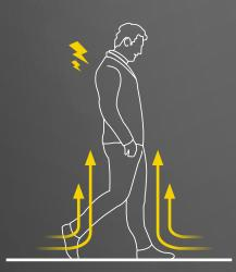
ESD is formed, for example, when walking. The human body is charged, so to speak, while doing so. The body can absorb high charges.
