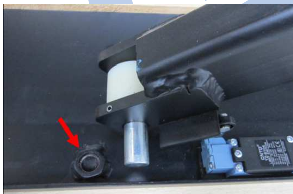
Figure 8 Installation of transport bolt 1
