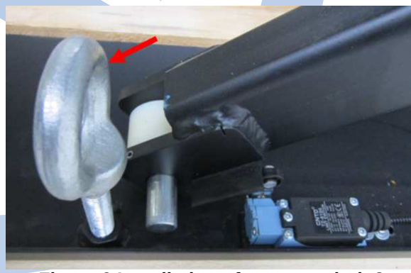
Figure 9 Installation of transport bolt 2
