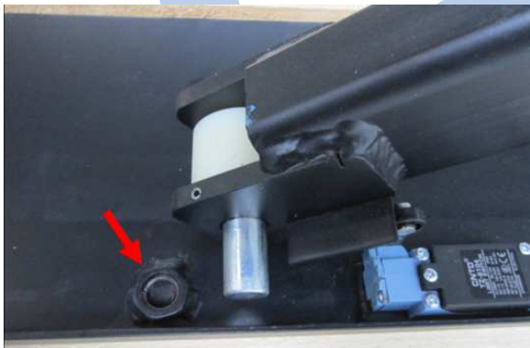
Figure 8 Installation of transport bolt 1
