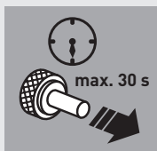
Fig. 3d: Waiting and releasing the throttle knob
