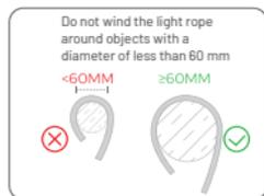
**EN** Incorrect use of the light rope can cause individual diodes to become unstable or stop glowing. However, this does not affect the overall performance of the product and a long lifespan can be ensured by avoiding violent pulling and hard twisting of the light rope.
