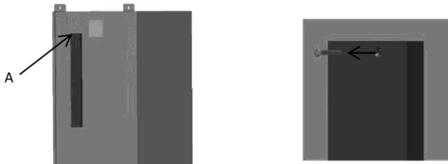
3. Screw the plinth cover onto the doubling from the front using the countersunk screws A from point 2 and the accessory pack.
