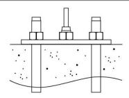
2. Hammer down and tighten the expansion anchor.
