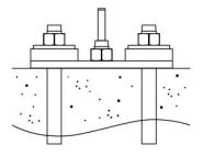
3. Unscrew the nut and provide 2 pcs expansion anchor with pu-spring, washer and locking nut. Tighten the locking nut to good contact to the washer.
