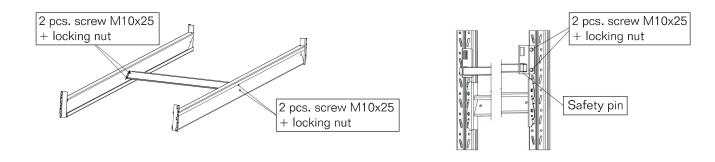
Beam L=3600mm with bracing gets increased capacity from 4x800 kg to 4x1000 kg.
