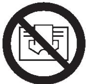
**WARNING:** In order to avoid overheating, do not cover the heater. Do not hang anything on the heater and do not cover it while it's working.
