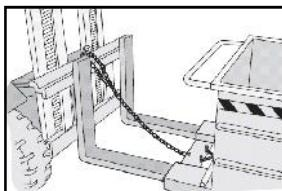
Connect the safety chain of the skip tilting container to the front crossbar of the fork carrier
