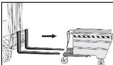
Place the forks into the appropriate fork jackets positioned on the bottom of the skip tilting container
