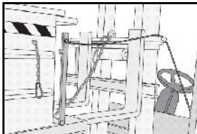
Place the release lever rope near the driver's seat
