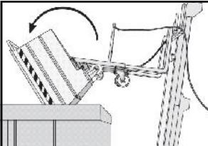
To unload the container: lift the skip tilting container just over the scraps collection container. Move forward with the fork lift truck until the skips tilting container is overlayed to the collection container. To unload the scraps pull the rope in in order to operate the release lever of the container
