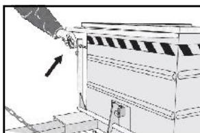
Remove the safety carabiner from the release lever of the container
