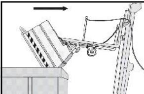
Move back in order to overlay the skip tilting container to the edge of the container
