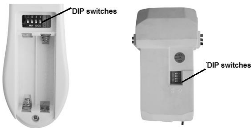
Fig. 11 Remote battery compartment
