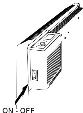
Use the Power / Stand-by button to turn the convector on and off without losing the stored time.
