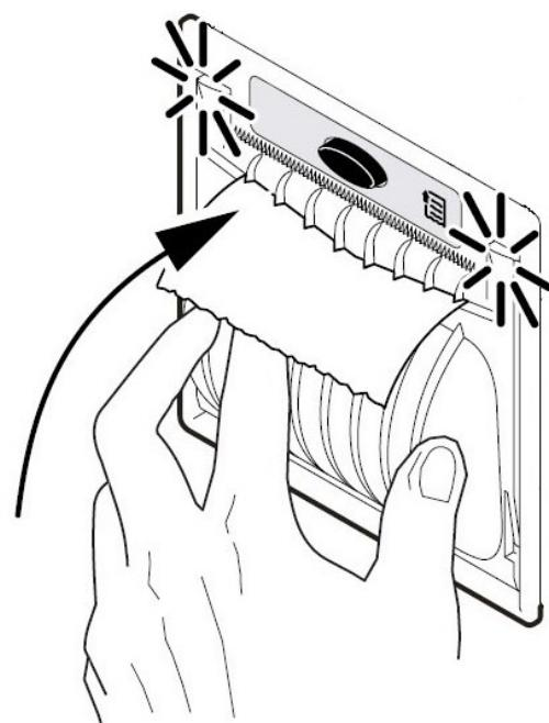
24.) Remove the excess of paper using sharp and higher edge.
