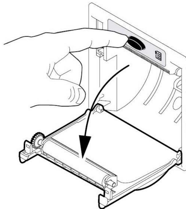
22.) Unroll a bit of roll of paper and placed it in correct position (beginning of roll backwards and up high) as on picture.
