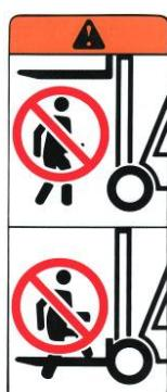
It is generally prohibited to linger underneath forks or any other attachments. Regardless of whether these are loaded or unloaded.
