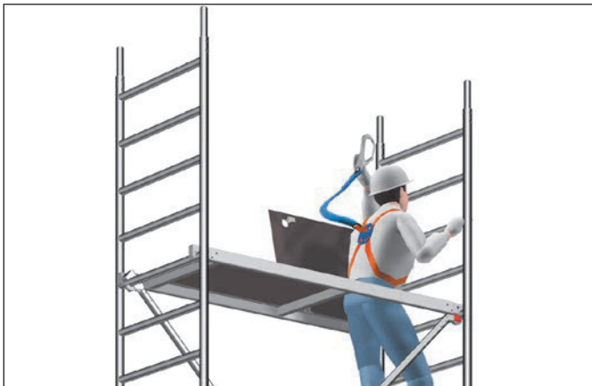
Fig. 1: Attachment of PSA during ascent to the unsecured level
