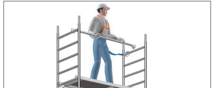
Fig. 3: Safe fitting of guardrails with PSA
