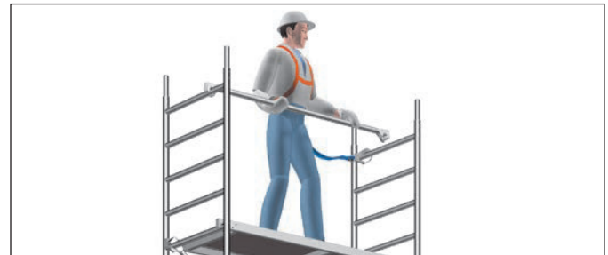
Fig. 3: Safe fitting of guardrails with PSA
