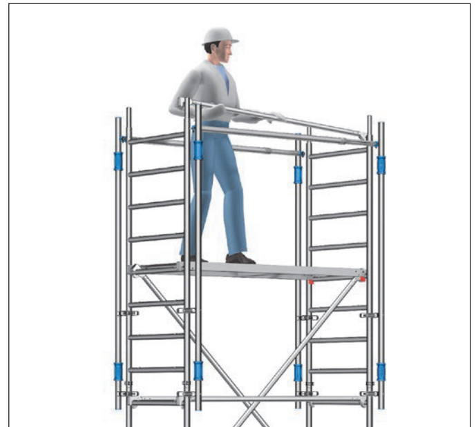
Fig. 6: Safe fitting of the guardrails with AGR
