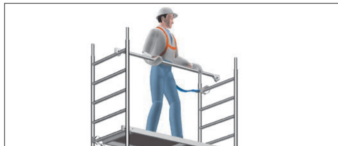
Fig. 3: Safe fitting of guardrails with PSA
