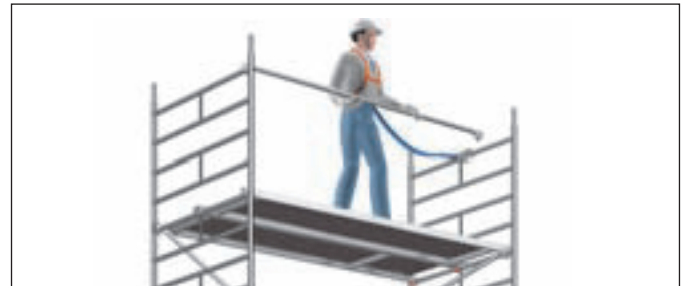
Fig. 3: Safe assembly of rear guardrails using PSA
