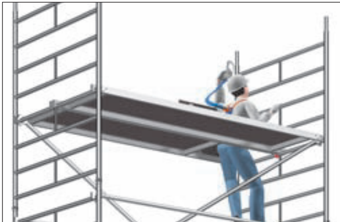
Fig. 1: Attachment of PSA during ascent onto the unsecured level
