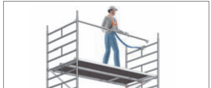
Fig. 3: Safe assembly of rear guardrails using PSA
