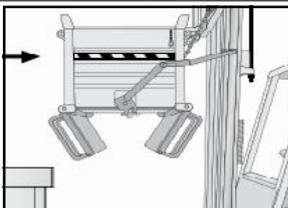
Move back until the container is out from the discharge zone.
