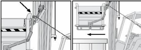
Place the release lever rope near the driver's seat. Lift the container about 10 cm from the ground. Move to the unloading area. Lift the container with openable bottom just over the scraps collection container. Move forward with the fork lift truck until container is overlayed to the collection container.
