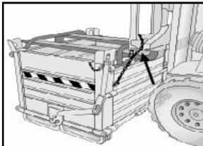
Connect the safety chain of the container to the front crossbar of the forklift truck.
