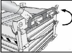
Lift upwards the external handles of the container.
