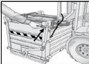
Remove the safety carabiner from the release lever for the bottom opening.
