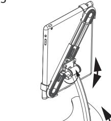
**△**To secure the tablet, tighten the holder thanks to the back screw.
