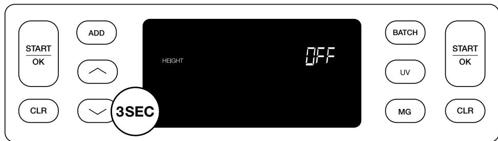
Please note that in this setting the device will not be able to detect banknotes of a different height and/or width when these are included in the counted stack.
