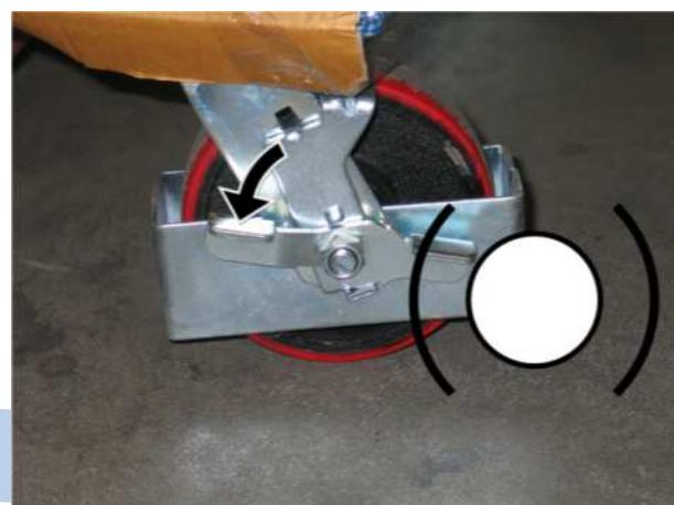
Figure 4 Release brake
