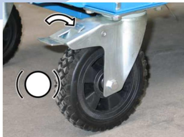
Figure 8 Release brake
