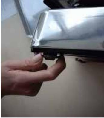
Level balance with foot screws until the air bubble of the water balance is in the prescribed circle.
