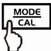
⇒ Remove all loads from the balance, press **TARE** and press repeatedly the **MODE** key until „PtArE“ flashing appears.
